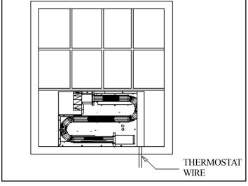
K.) Locate factory installed thermostat wires extending from the front of heater. Connect 24 V. wall thermostat (provided) to heater using a maximum 20' of thermostat wire. Do <u>not</u> splice thermostat wire. (See Figure 9).
